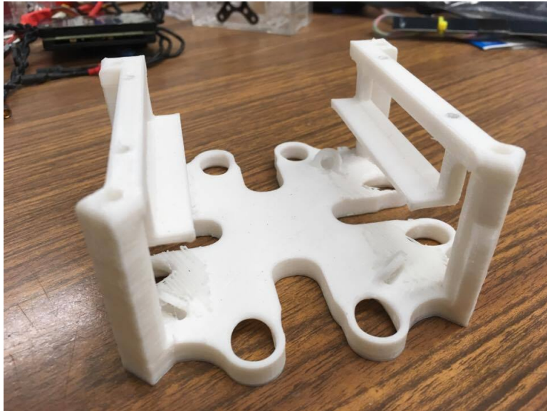
Figure 5.3: The 3D-printed frame that holds the electronics.
