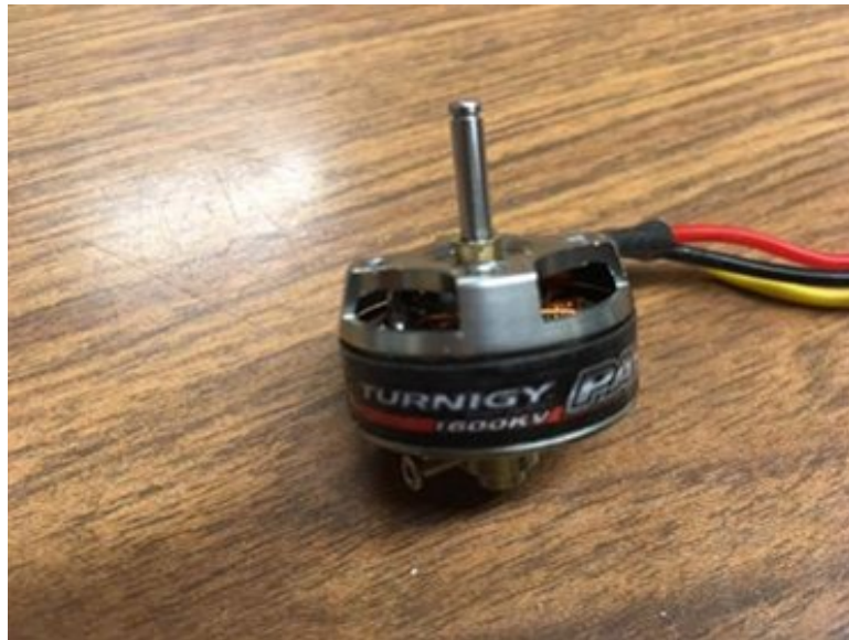
Figure 5.9: One of the Turnigy Park 300 1600kv motors used.
