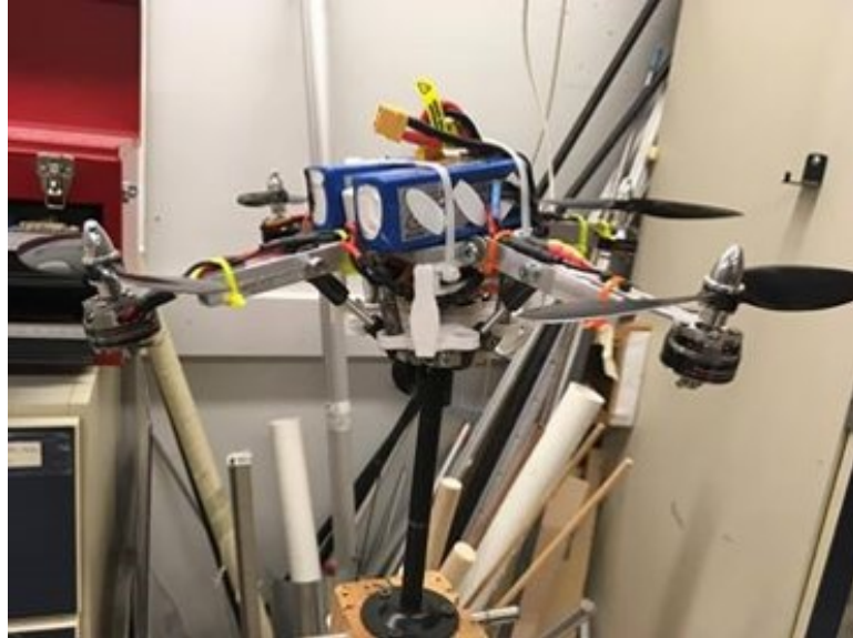
Figure 5.10: The quadrotor on the test rig for thrust measurements.
