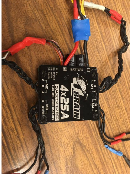
Figure 5.11: The QBrain ESC hub that regulates the voltage to the motors.
