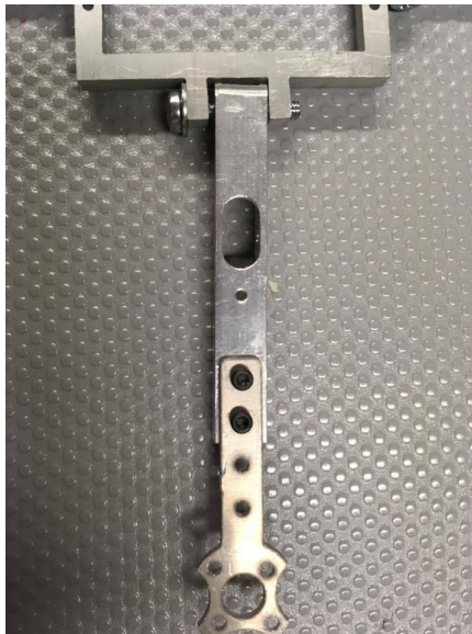
Figure 5.8: One of the four arms of the quadrotor with the motor mount attached.
