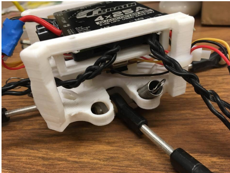
Figure 5.4: A side view of the frame showing how the springs line up.
